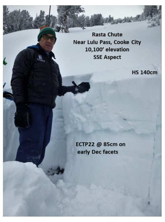
A layer of facets that formed in early December is breaking clean in stability tests (ECTP22) about 1.5 feet under the surface. Wind-loading or more snow will make this layer more reactive. Photo: GNFAC
