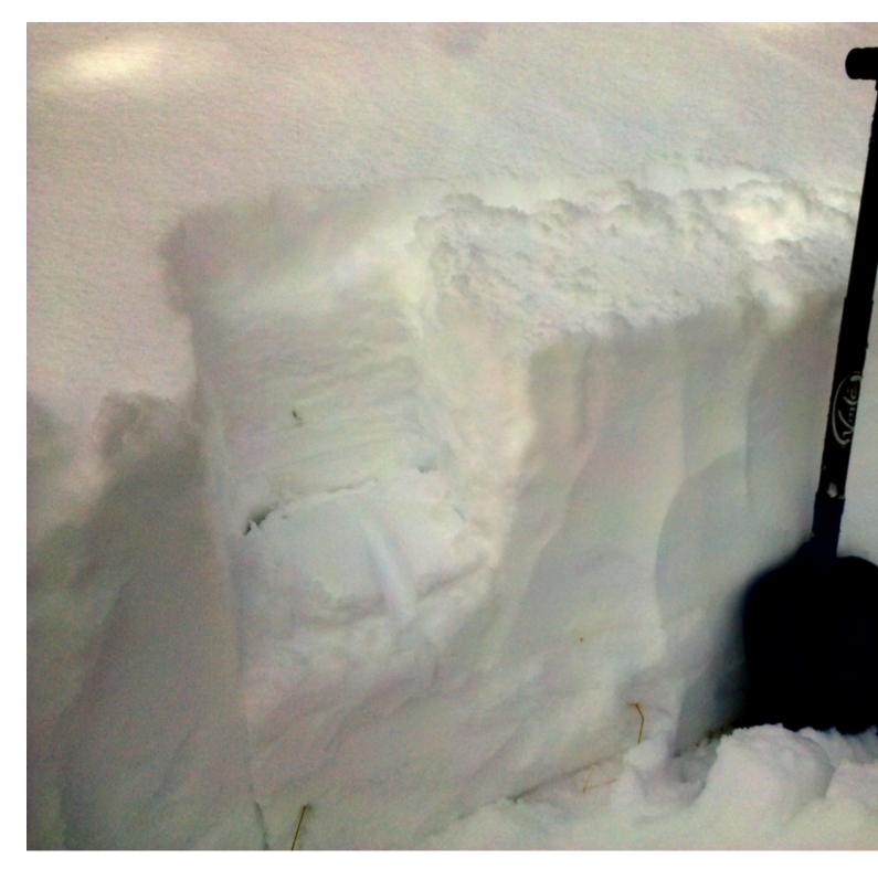
This photo was taken in the northern Gallatin Range, west of Hyalite Canyon, at 6900 ft on an east facing, 35 degree slope. This extended column test produced no fractures. For this time of year at 6900 ft this is an exceptionally deep snowpack and promises a good foundation for the rest of the season. Photo: T. Gerling
