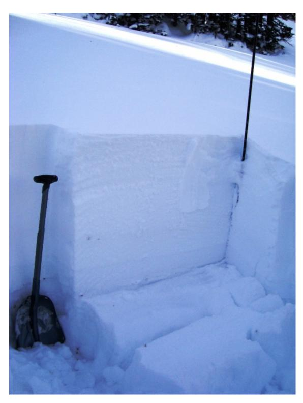
This 115cm deep pit was dug on an east aspect at 9,100 feet near Hyalite Lake. The ECT failed on 21 taps, twice, and broke clean indicating unstable conditions. It is breaking on 5 cm of sugary facets sitting on an ice crust. Cracking, collapsing and avalanches were seen on this layer in the last 48 hours. Photo: GNFAC
