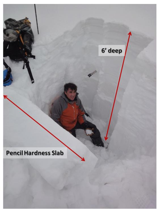
This pit was dug on a northwest facing slope at 8,750' in Lionhead. A dense, six foot thick pencil hardness slab is being supported by fist hardness depth hoar. I scooped out some in my hand. The column broke on this layer and I was able to lay the pillar, intact, outside the snowpit. The deeper the depth hoar gets buried, the more difficult it becomes to trigger. But if you get unlucky and trigger it the avalanche will be large, destructive and deadly. Photo: GNFAC
