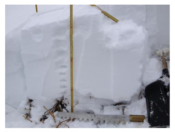
Bridger Bowl Snbow Safety dug this pit near the top of Pierre's Knob lift. They got collapsing on the layer of facets near the ground as they skied. Test score on the column were ECTP18 breaking 12 cm from the ground. Photo: P. Maleski
