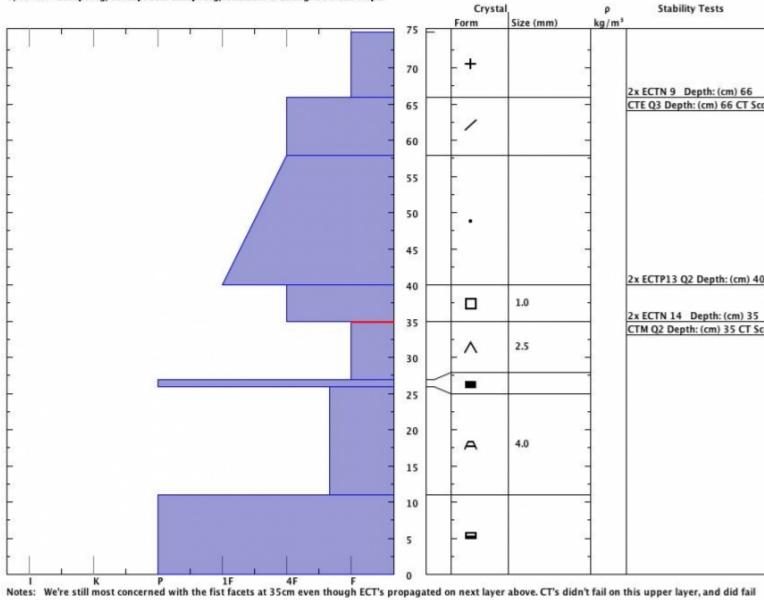
tes: We're still most concerned with the fist facets at 35cm even though ECT's propagated on next layer above. CT's didn't fail on this upper layer, and did fail on the fist facets. Several large collapses and shooting cracks ocurring on fist facets. We felt nervous on slopes above 27-28 degrees (measured).
