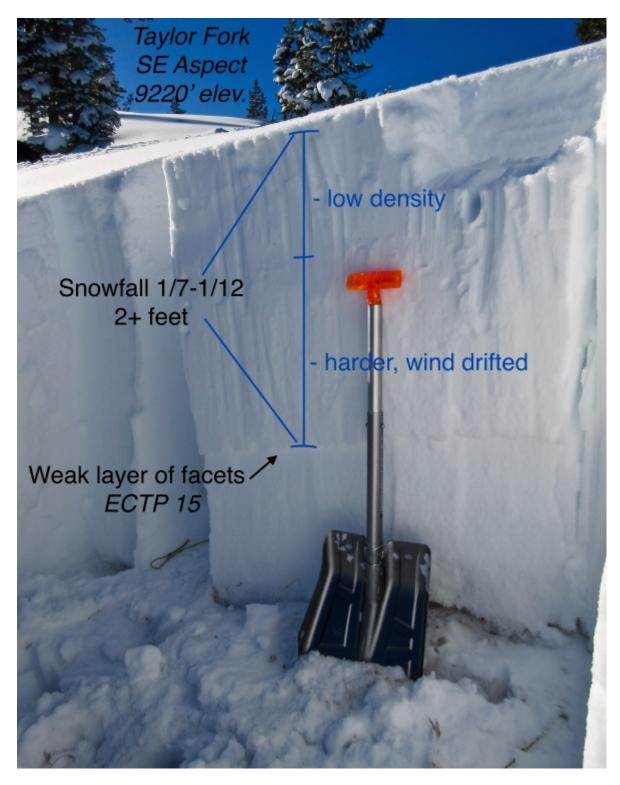
A thin weak layer of facets that formed during cold temperatures are buried by last week's 2+ feet of snowfall. We found unstable test results in this pit, and the poor structure makes avalanches possible to trigger on this layer. Photo: GNFAC
